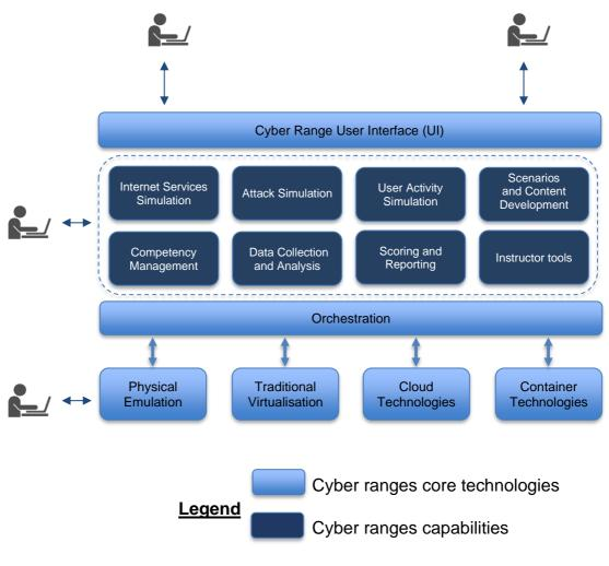
Figure 1 – Sample Architectural Components of a Cyber Range
